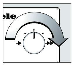
■ Set the roller speed selector to the desired speed.
